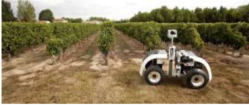
Fig. 5. Vine Robot, a prototype of an autonomous navigation robot used for vineyard monitoring, has been developed in Europe ( www.vinerobot.eu ).
