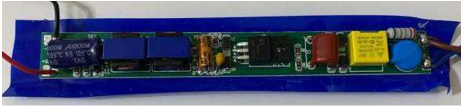
Figure 2.16 Micro Sprout Plant Growth Armature Driver
